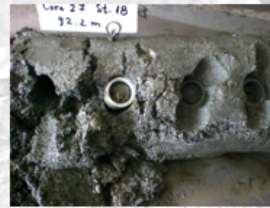
Optically Stimulated Luminescence (OSL) dating samples being taken.
